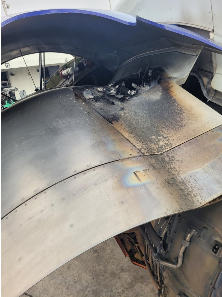
Figure 1 - Burned area above borescope port M. (Source: Atlas Air.)
